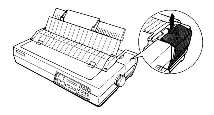
2. Plug the Multi-Font Module carefully into either Slot A or B. The arrow on the module should point toward the printer.
